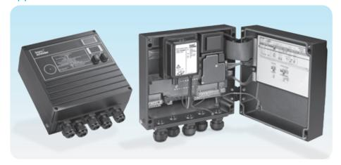
The BCU unites the functionally inter-related components of automatic burner control unit, ignition transformer, Manual/Automatic mode and display of operating and fault statuses in a compact metal housing.
